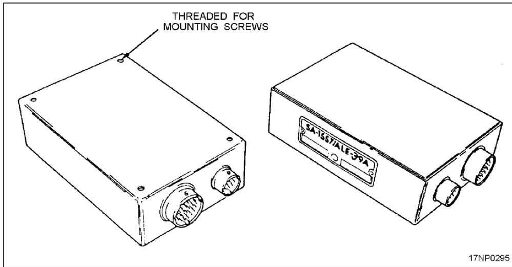
Figure 10-21.—Sequencer switch.
