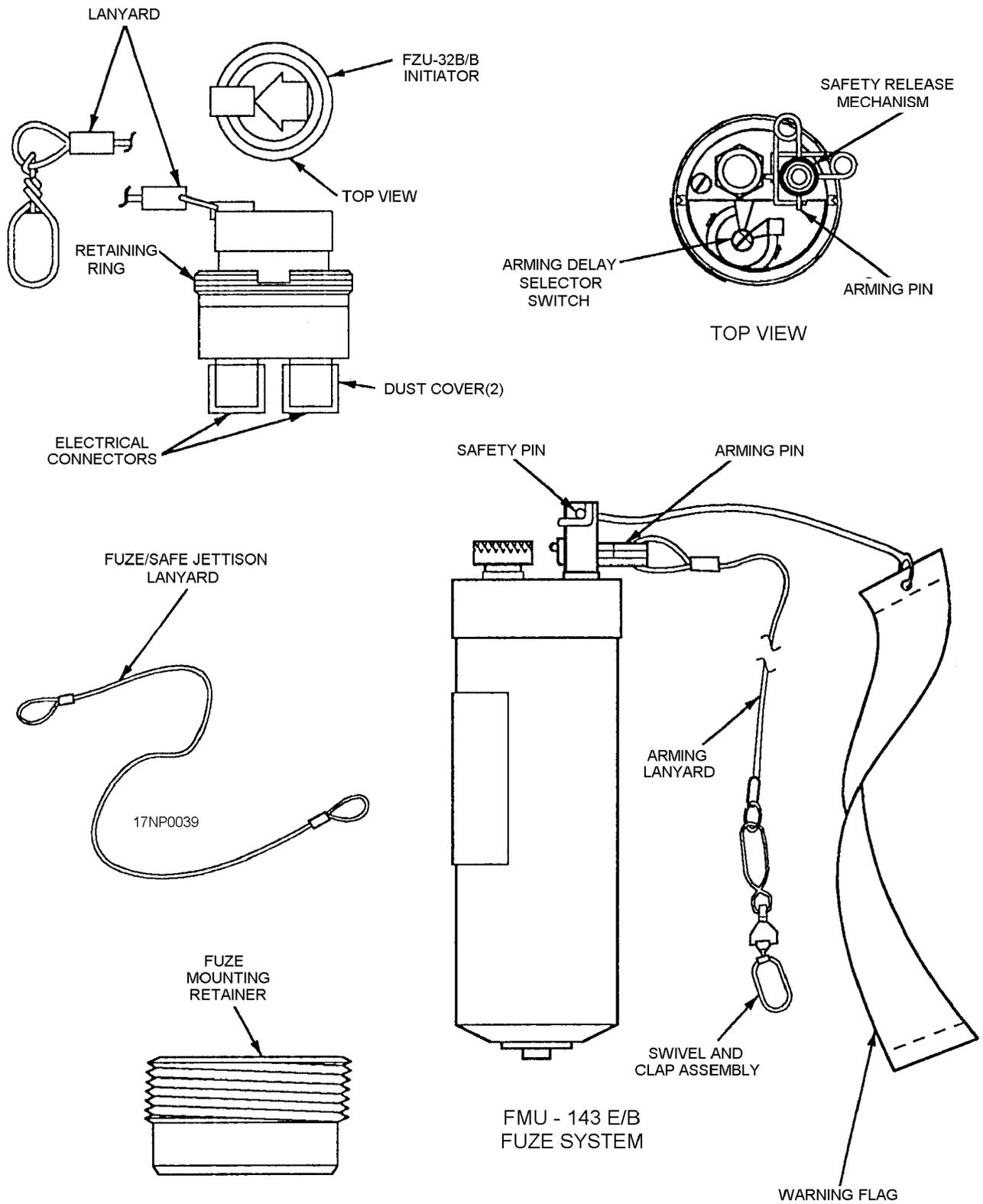
Figure 1-7.—FMU-143E/B electric tail fuze.
