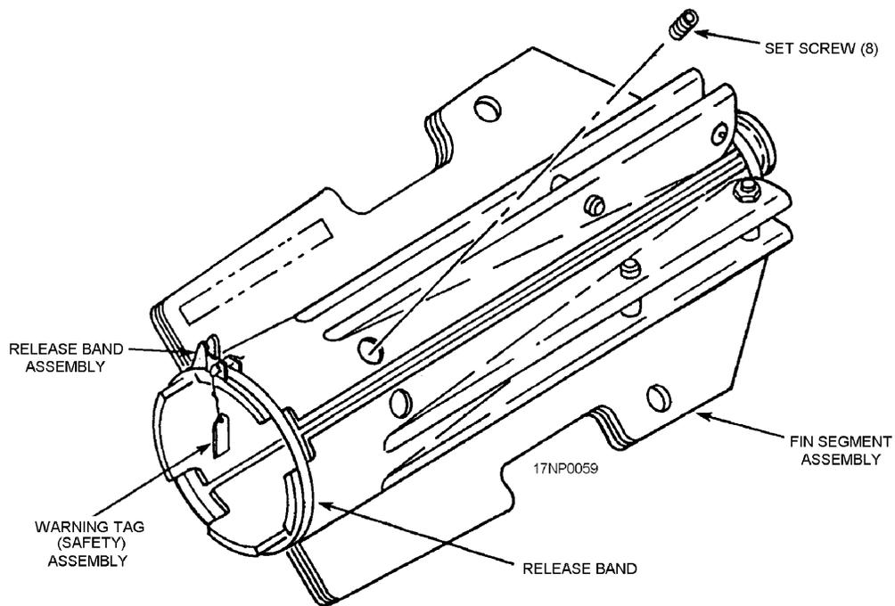
Figure 1-22.—Fin release band for Mk 15 fin.
