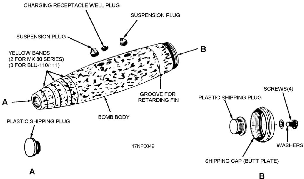
**Figure 1-15.—LDGP bomb Mk 80 (series)—exploded view (shipping configuration).**
