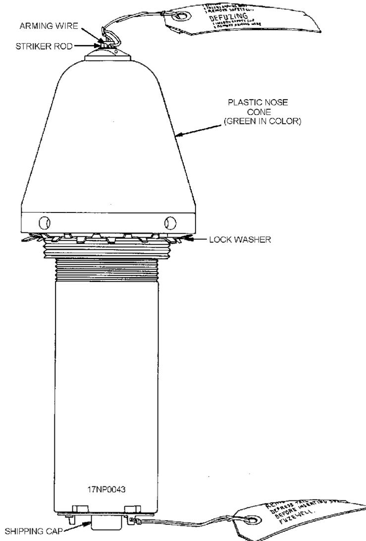
**Figure 1-11.—Mk 43 Mod 0 target detecting device.**
