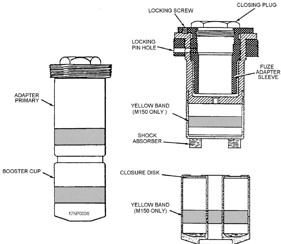
Figure 1-5.—Adapter-booster M150/T46 (series).
