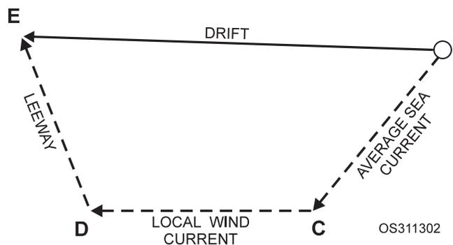
Figure 13-2.—Plotting drift.
