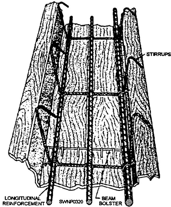
Figure 7-8.—Steel in place in a beam
