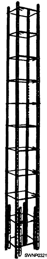
Figure 7-9.—Column steel in place.
