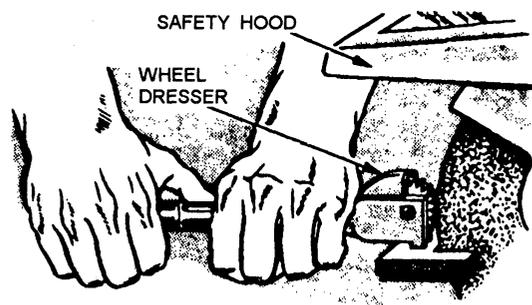
Figure 1-3.—Using a grinding wheel dresser.
