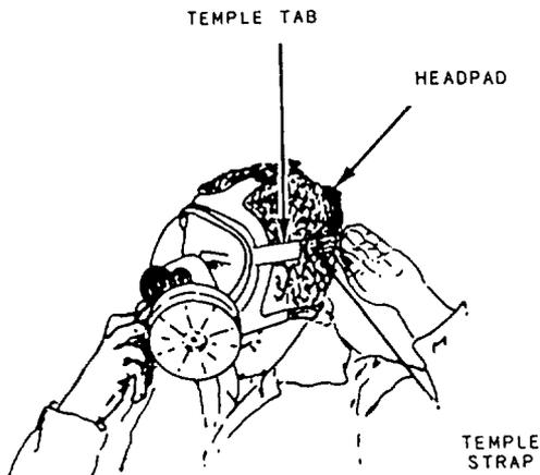
8. Tighten one temple strap (fig. 6-7) until the mask feels snug on that side. Tighten the other temple strap until both sides feel the same. (Tighten all straps toward the rear of the head with small jerks vice a long pull.)
