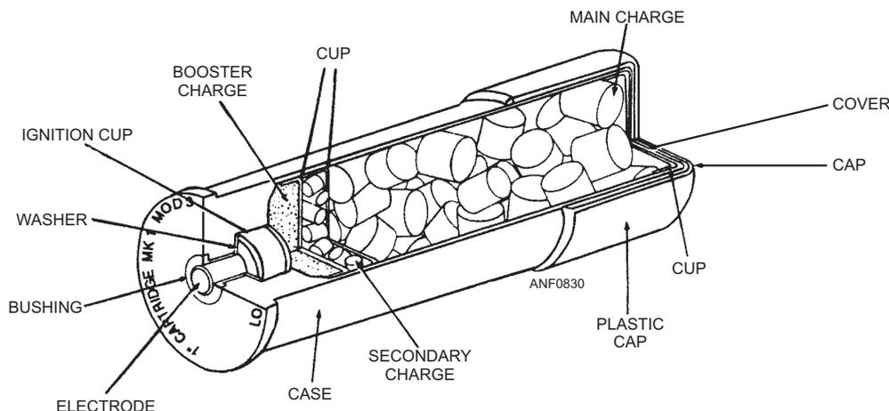
**Figure 8-30.**—Mk 1 Mod 3 impulse cartridge (sectioned).
