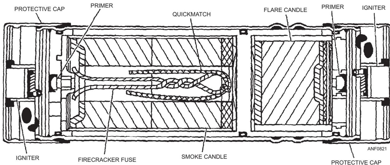
Figure 8-21.—Mk 124 Mod 0 marine smoke and illumination signal.
