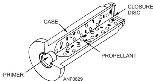
**Figure 8-29.**—Mk 97 Mod 0 impulse cartridge.
