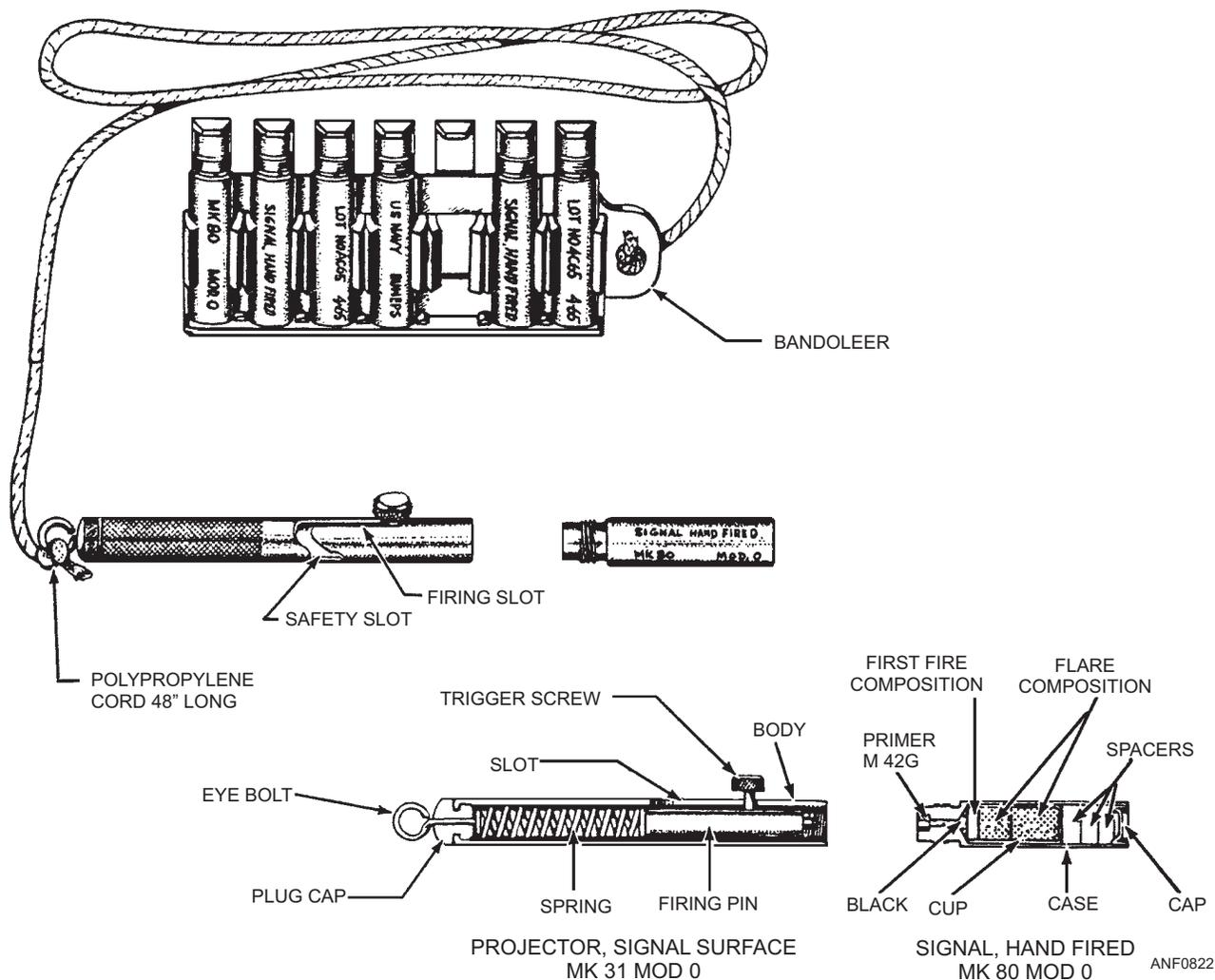
Figure 8-22.—Mk 79 Mod 0 illumination signal kit.
