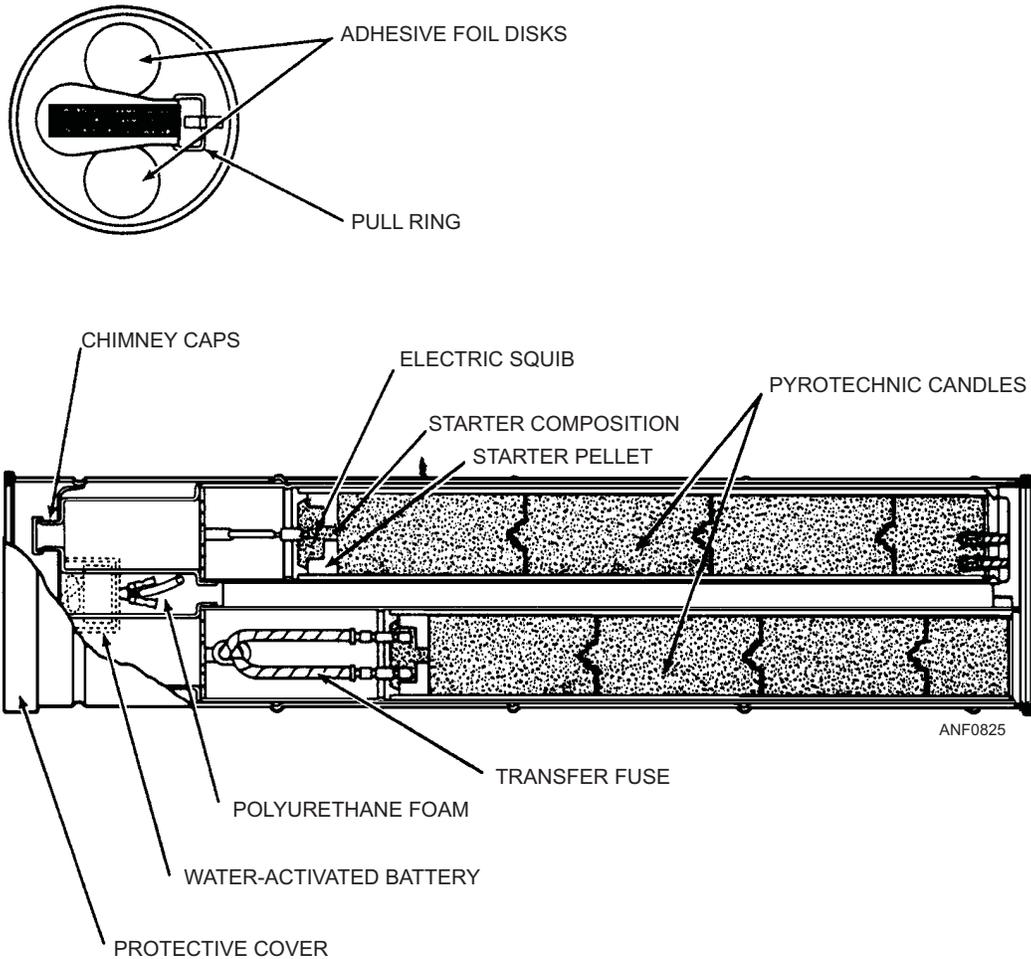
Figure 8-25.—Mk 58 Mod 1 marine location marker.
