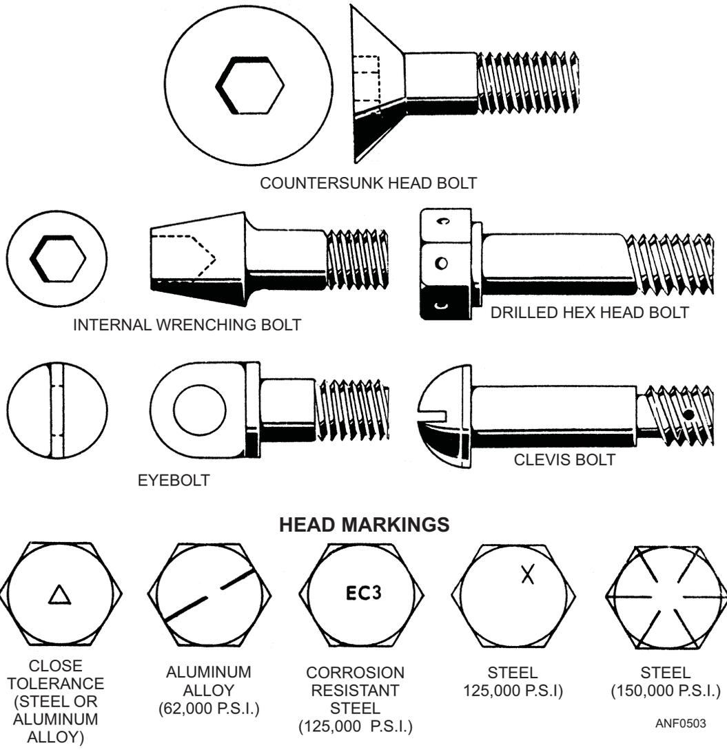
Figure 5-3.—Types of bolts and bolt head markings.
