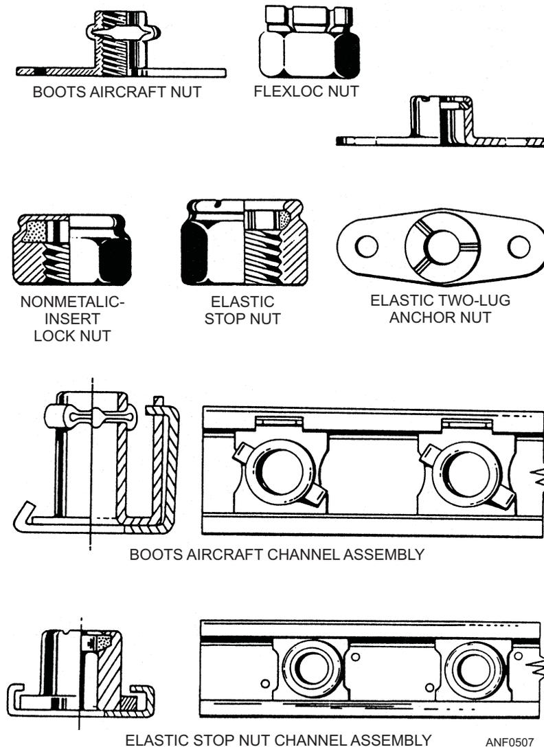
Figure 5-7.—Self-locking nuts.
