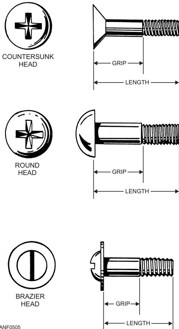
Figure 5-5.—Structural screws.
