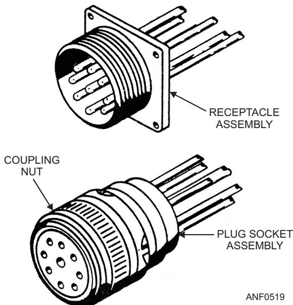
Figure 5-19.—Connector assembly.
