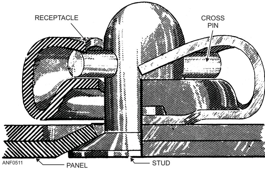
Figure 5-11.—Airloc fastener.
