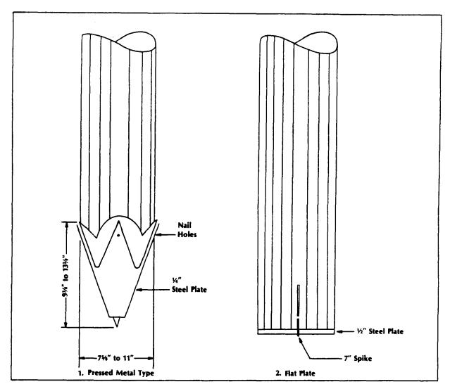
Figure 4-1 Steel shoes for timber piles
