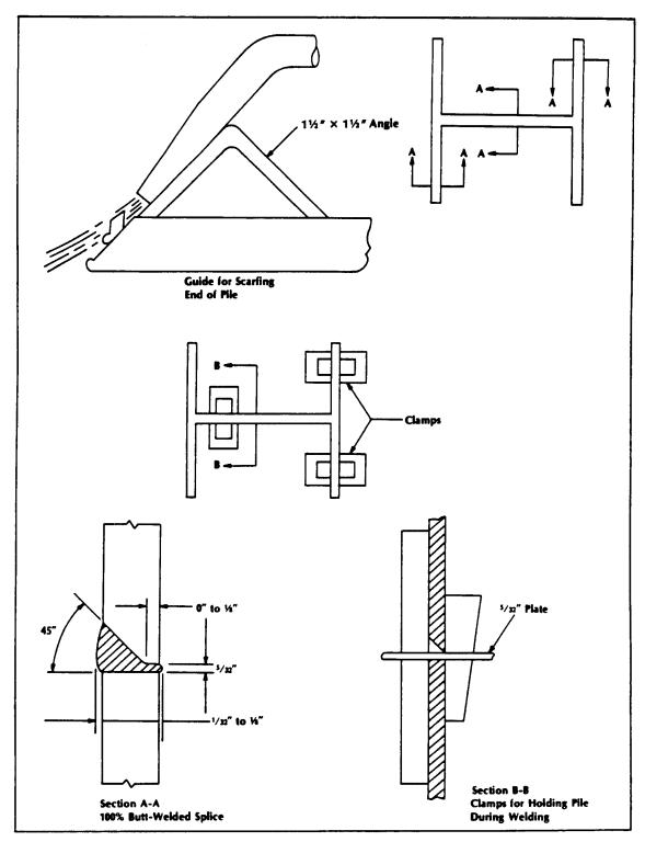
Figure 4-5 Butt-welded splice, welding clamps, and guide for scarfing
