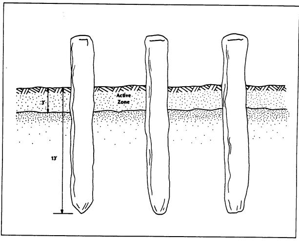
Figure 4-22 Piles driven through 3 feet of active zone to a depth of 13 feet after thawing
