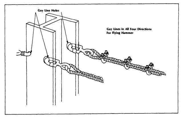
Figure 4-9 Method of guying steel piles
