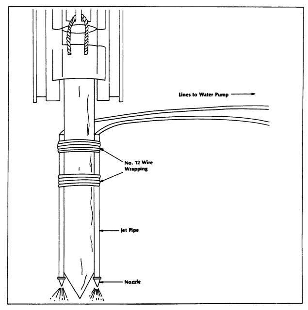
Figure 4-14 Use of jet pipes near pile tip
