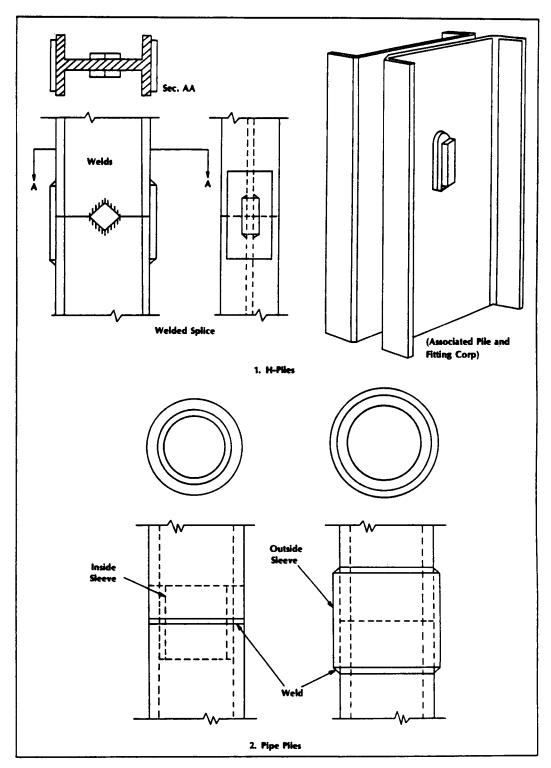
Figure 4-6 Splices of H-piles and pipe piles
