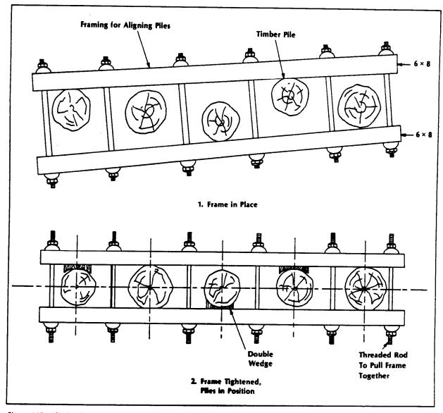
Figure 4-19 Aligning frame for pile bent
