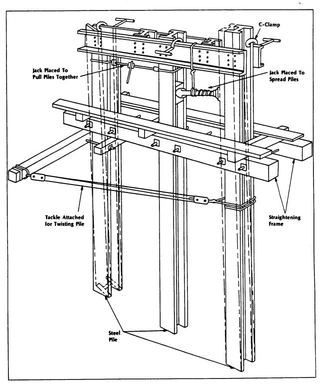
Figure 4-20 Aligning and capping steel pile bents
