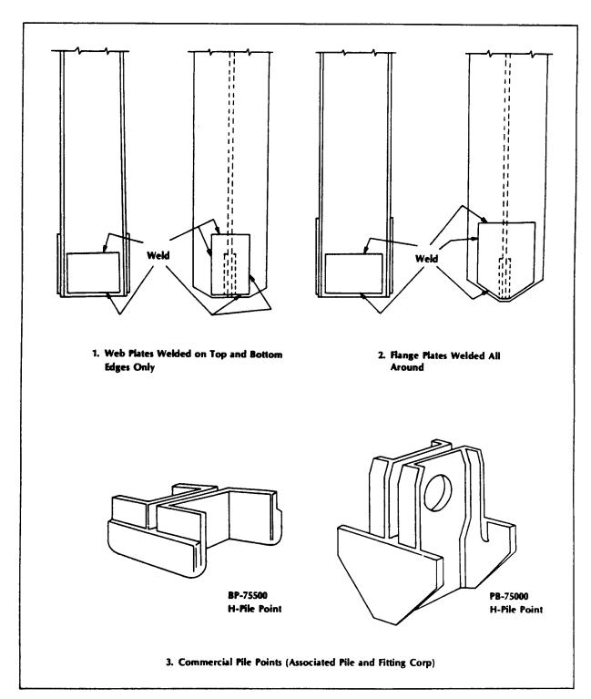
Figure 4-3 Driving points for H-piles
