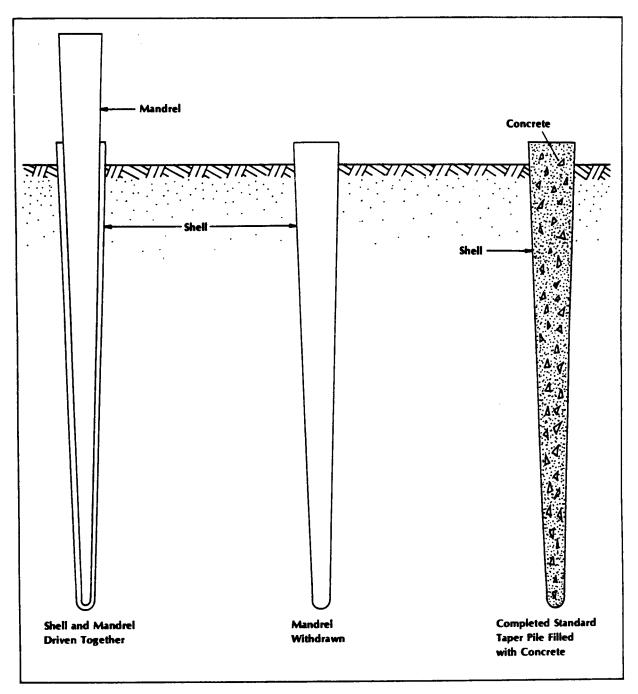
Figure 4-25 Procedure for placing shell-type, cast-in-place concrete piles
