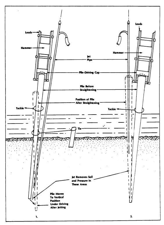
Figure 4-16 Realigning piles by jetting
