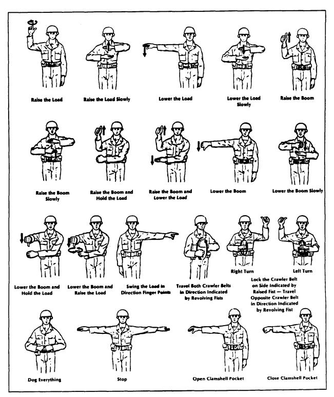
Figure 4-26 Hand signals for pile-driving operations
