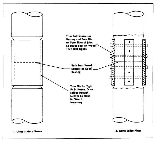
Figure 4-2 Methods of splicing timber piles
