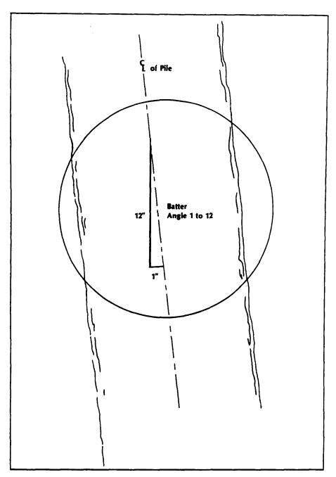
Figure 4-10 Batter of a pile
