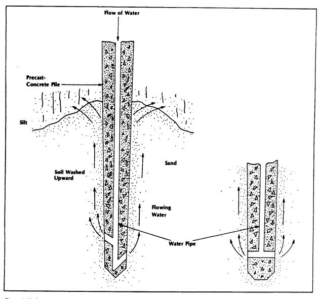
Figure 4-15 Precast concrete piles with internal jetting pipes
