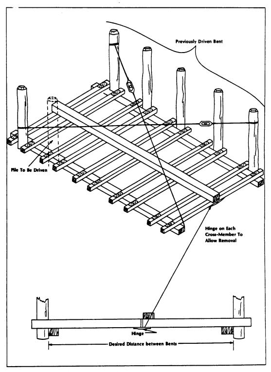
Figure 4-18 Floating template for positioning piles
