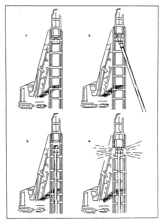
Figure 4-7 Basic steps in setting and driving piles
