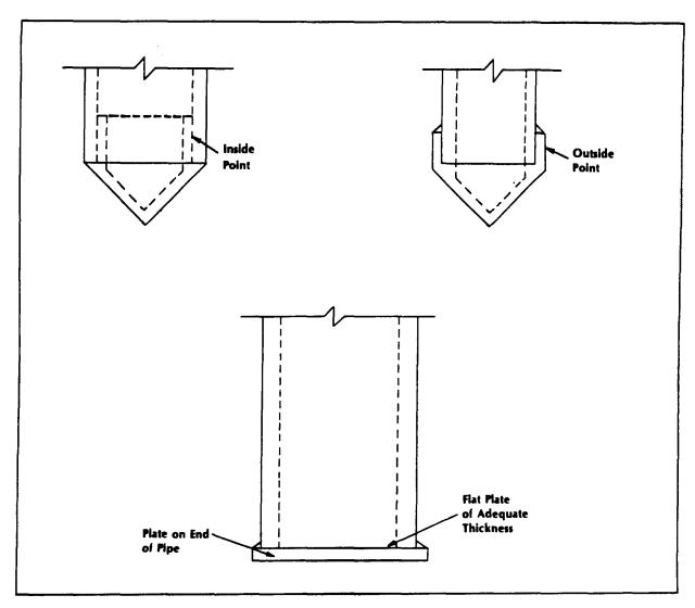
Figure 4-4 Driving points for pipe piles
