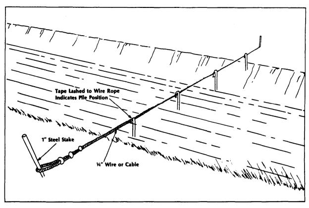
Figure 4-17 Wire rope guideline to position piles
