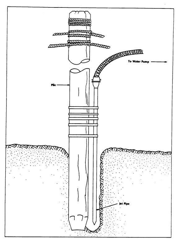
Figure 4-13 Jetting pile by pipes and hoses
